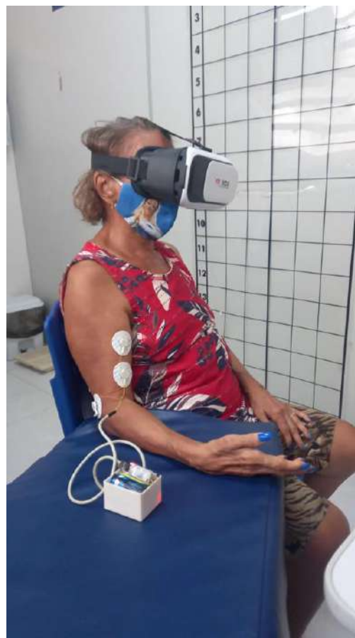
Fig. 3 Positioning the patient, electrodes and VR goggles during collection using the developed equipment.
