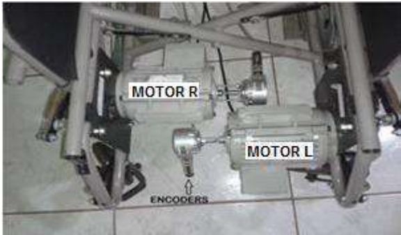
Figure 4.:Motor's A.C MIT installed in- Wheelchair By:The authors
