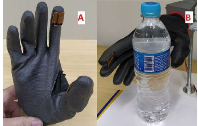
Fig. 2: Piezoresistive sensor array. A) Sensor array placed on the prosthesis indicator. B) Prosthesis holding bottle and showing positioning of sensors in the experiment.
