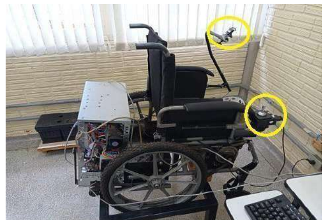
Figure 1.: Prototype with manipulators, blow and suction, and joystick in yellow
