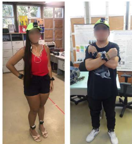
Fig. 9 Visually impaired volunteers wearing assistive navigation device with WBAN for testing.
