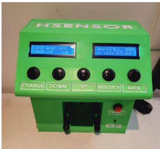
Fig. 2: Photograph of the developed mechanical stimulation equipment designed to replicate the mechanical conditions of knee articular cartilage, demonstrating its functionality and robustness as proposed.
