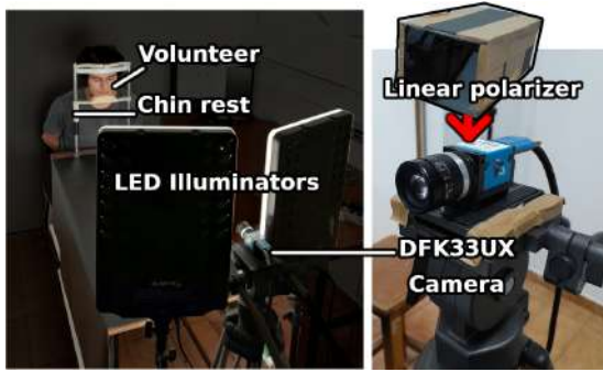
Fig. 1: Experimental setup for video acquisition. The box with the linear polarizer attaches to the top of the camera.
